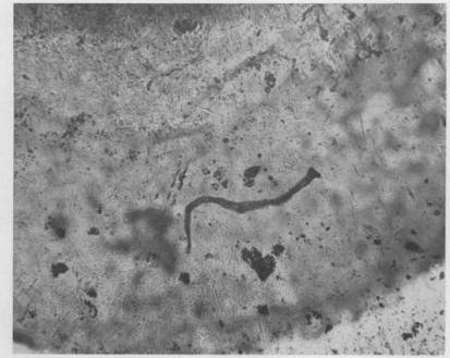
MICROSCOPIC DEBRIS on an electrical contact looks like this when magnified 108 times. The snake-like object in the center is a minute nylon fiber about 1/50th of an inch long. Other spots are metallic dust and foreign materials. Microchemists of 1621-3 detect and identify the debris and find means of avoiding it in the production of electrical contacts necessary for various components.
